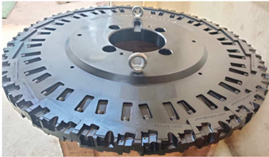
Ø800MM external pin milling cutter
